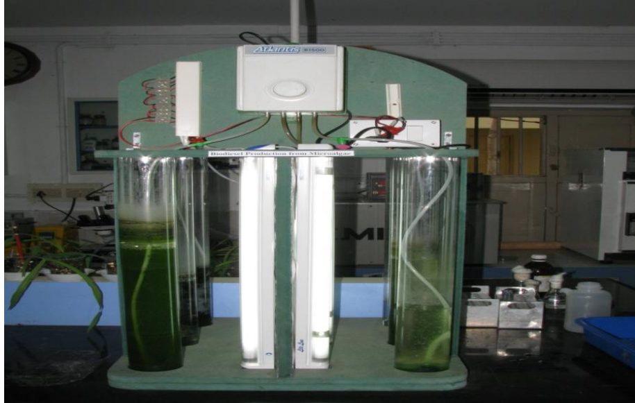
Fig.7. Photobioreactor for algae cultivation (30L capacity)
